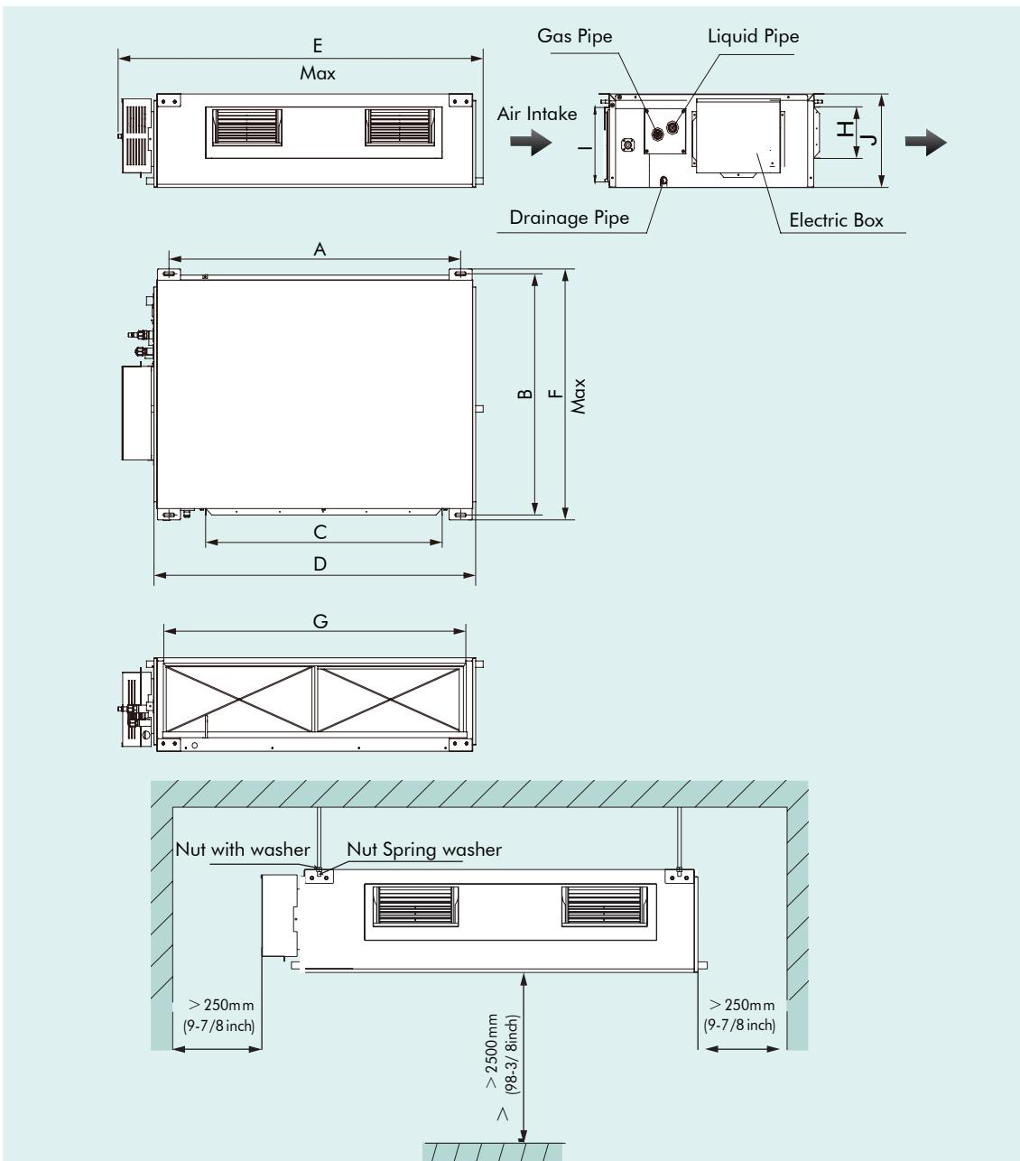
Note: The condensate drain line should be installed with a minimum of 5° slope to ensure proper drainage.
